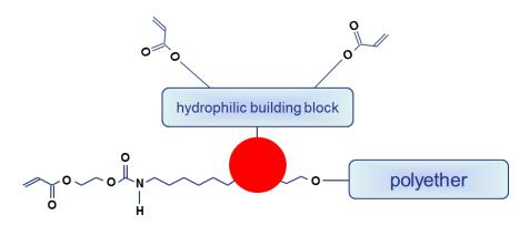
Figure 5. Water dilutable urethane acrylate
