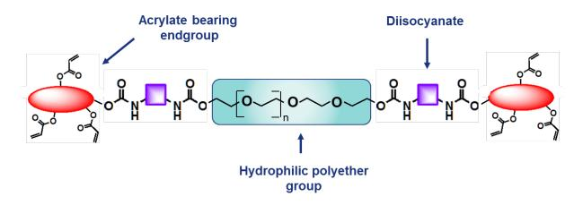
Figure 2. Schematic representation of a typical water thinnable UV curable polyurethane resin.
