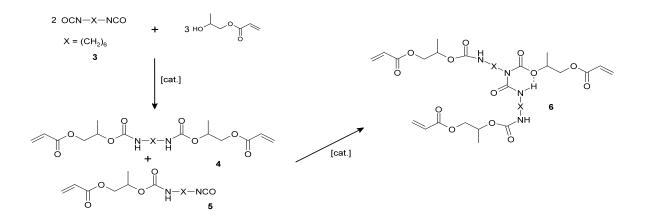
Figure 3. Direct allophanatisation without distillation step.
