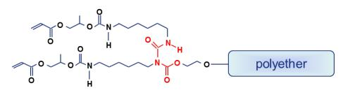
Figure 4. Water compatible allophanate based urethane acrylate.
